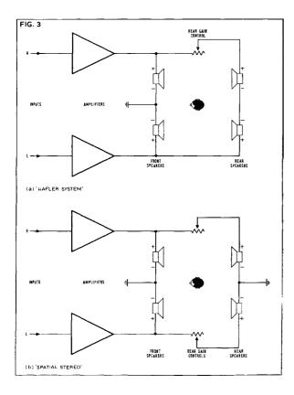
volume can be independently adjusted; or alternatively, a variable resistor can be placed in series with the rear speakers to provide volume adjustments, as in Fig 3(a).
