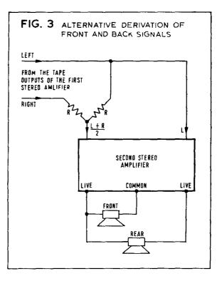
A central mono sound (*eg* a mono disc played with the equipment switched to stereo) should then be played over the system, and the balance control of the second amplifier should be carefully adjusted to minimise the output of the rear speaker. Once this is done, the rear speaker should reproduce the difference of the two stereo channels, and the balance control of the second amplifier should thereafter be left untouched.
