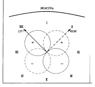
speaker set-up. A sound from position II of Fig 5 will only be picked up on the right-channel, so will be reproduced to the right of the listener. A sound from position III of Fig 5 will be picked up as an out-ofphase stereo signal, so will be reproduced from behind the listener. Similarly, sounds from positions IV, V, VI, VII and VIII of Fig 5 will be reproduced, respectively, to the left, front, right, rear and left of the listener.
