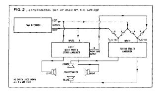
The above arrangement has the disadvantage that it can only be used with high level unequalised programme sources such as tape or radio. Those who are capable of constructing phase inverters (or have transformers which can be used as phase inverters) can also use low-level and equalised sources (such as disc) by deriving the signals for the second amplifier from the tape outputs of the first amplifier, which need not then be a Quad. The advantage of the above
