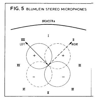
speaker set-up. A sound from position II of Fig 5 will only be picked up on the right-channel, so will be reproduced to the right of the listener. A sound from
